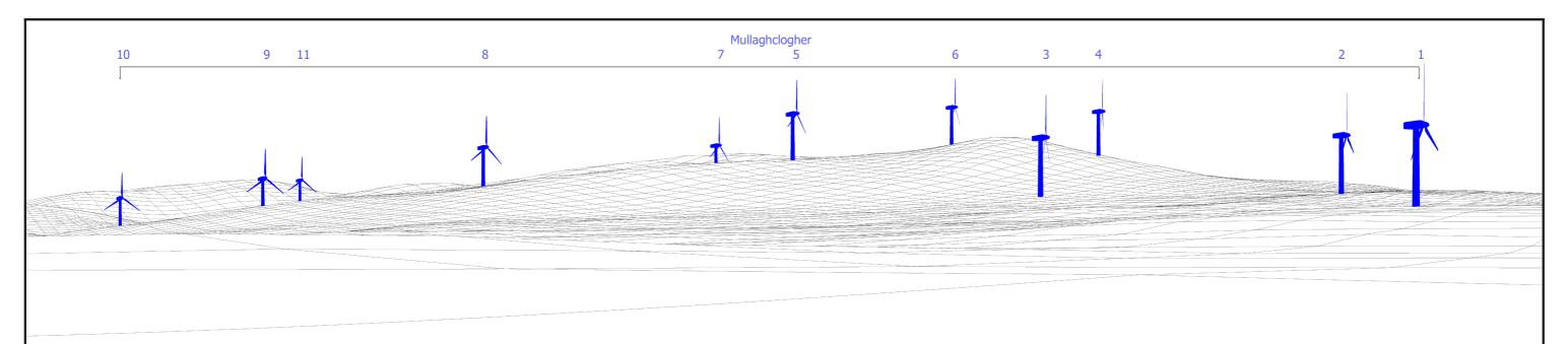
**Notes:** Mullaghclogher turbines shown in blue. Turbine dimensions illustrated: 180 m max. tip height above ground level; 150 m rotor diameter; 105 m hub height Where present in view: Existing wind farms in red; Consented wind farms in orange; Proposed wind farms in green; Single turbines may also be visible in the baseline photography.
