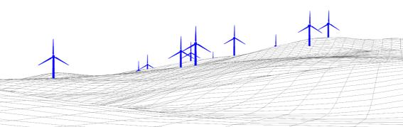
**Notes:** Mullaghclogher turbines shown in blue. Turbine dimensions illustrated: 180 m max. tip height above ground level; 150 m rotor diameter; 105 m hub height Where present in view: Existing wind farms in red; Consented wind farms in orange; Proposed wind farms in green; Single turbines may also be visible in the baseline photography.
