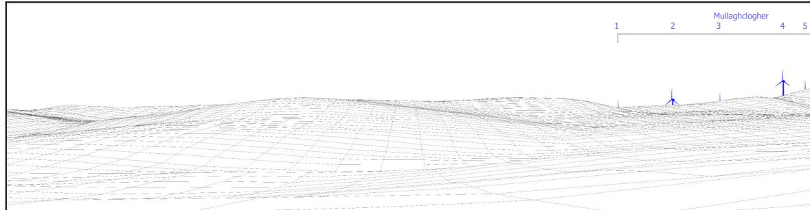
**Notes:** Mullaghclogher turbines shown in blue. Turbine dimensions illustrated: 180 m max. tip height above ground level; 150 m rotor diameter; 105 m hub height Where present in view: Existing wind farms in red; Consented wind farms in orange; Proposed wind farms in green; Single turbines, which may also be visible in the baseline photography.
