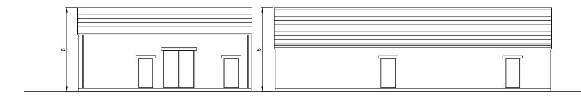
SUBSTATION CONTROL BUILDING ELEVATION A SCALE 1:250
