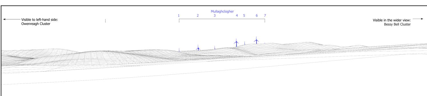
Notes: Mullaghclogher turbines shown in blue. Turbine dimensions illustrated: 180 m max. tip height above ground level; 150 m rotor diameter; 105 m hub height Where present in view: Existing wind farms in red; Consented wind farms in orange; Proposed wind farms in green; Single turbines, which may also be visible in the baseline photography.
