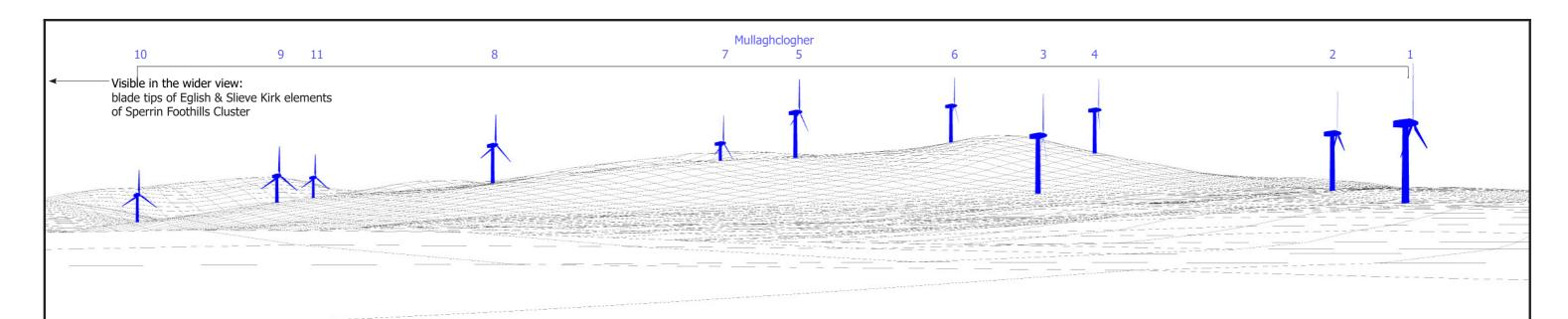
Notes: Mullaghclogher turbines shown in blue. Turbine dimensions illustrated: 180 m max. tip height above ground level; 150 m rotor diameter; 105 m hub height Where present in view: Existing wind farms in red; Consented wind farms in orange; Proposed wind farms in green; Single turbines, which may also be visible in the baseline photography.
