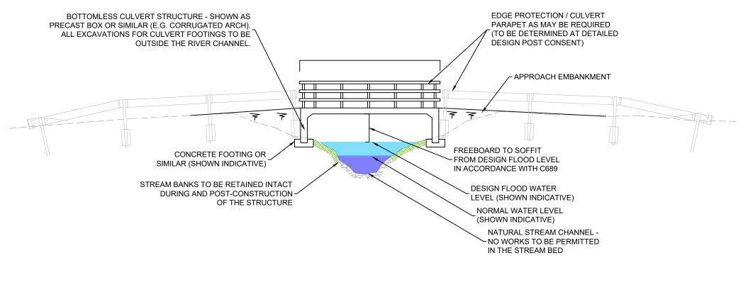
TYPICAL BOTTOMLESS CULVERT WATERCROSSING SCALE - 1:100
